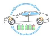
Regenerative braking, found in hybrid and full-electric vehicles, converts kinetic energy from braking into electrical power to charge the vehicle's high-voltage battery. Also known as a kinetic energy recovery system, it uses electric motors in reverse to act as generators. This system slows the car, aiding traditional brakes, improves fuel consumption, and reduces wear on brake pads by decreasing the overall braking load. winmeen.com 2024 JUL 12
