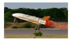
✓ ISRO achieved the third successful landing of its Pushpak reusable launch vehicle (RLV LEX-03), testing it under challenging conditions. The vehicle reused components from previous flights and employed advanced sensors for precise landing. Designed to reduce launch costs significantly, it aims to retrieve and land like an airplane after deploying satellites into space.
